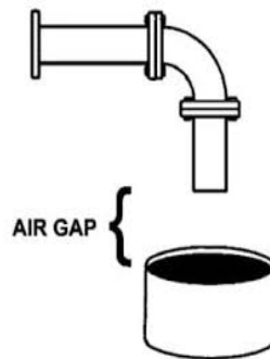
Figure 1. Air Gap Separation
